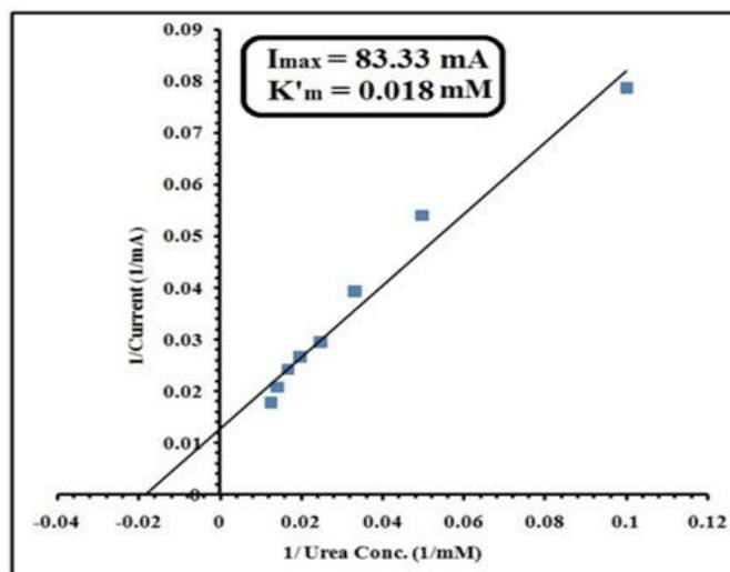
Figure 7: Lineweaver–Burk plot of PANI/ZnO/Urease Biosensor
