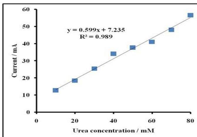
Figure 6: Calibration curve of PANI/ZnO/Urease Biosensor.
