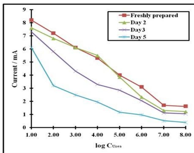
Figure 7: Storage stability of PANI/ZnO/Urease Biosensor.
