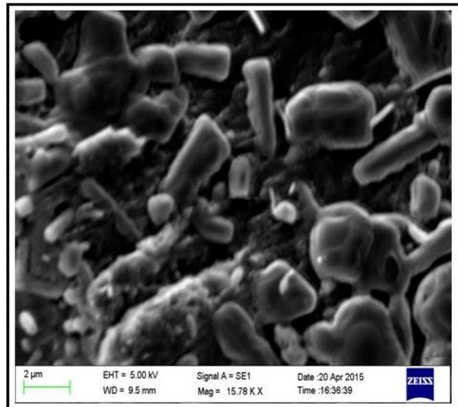
Figure 2: SEM image of Nanostructured ZnO.
