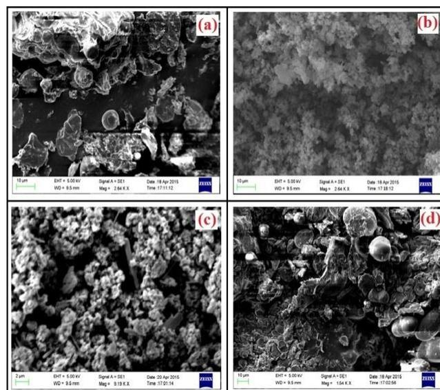
Figure 3: SEM image (a) Urease (b) Pure PANI (c) PANI/ZnO (d) PANI/ZnO/Urease.
