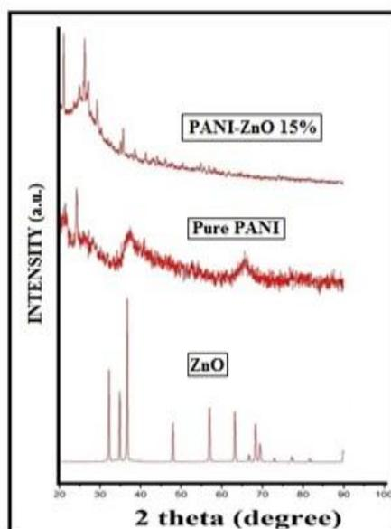
Figure 5: X-RD pattern of PANI/ ZnO nanocomposites
