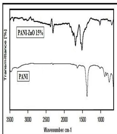
Figure 4: Relative IR peaks of PANI and PANI/ZnO nanocomposite
